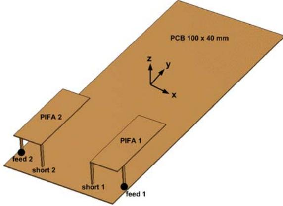
Fig. 1 3D View of the dual PIFA structure
