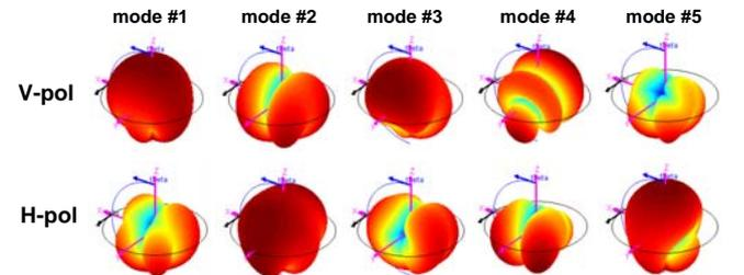
Fig. 6. Vertical (top) and horizontal (bottom) far field components of all the five modes at 2 GHz
