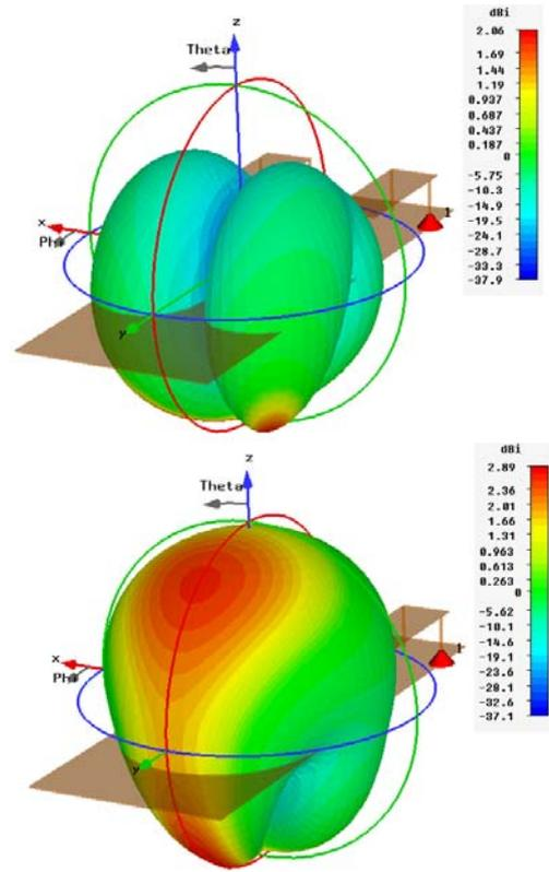
Fig. 8. Vertical (top) and horizontal (bottom) far field components at 2 GHz for out-of-phase excitation
