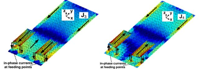
Fig. 4 Distribution of the characteristic currents  $J_3$  (left) and  $J_4$  (right) at 2 GHz
