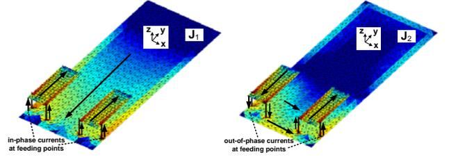
Fig. 3 Distribution of the characteristic currents  $J_1$  (left) and  $J_2$  (right) at 2 GHz
