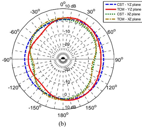
Fig. 9. Comparison of CST and TCM farfields cuts at 2 GHz (superposition of two modes for each polarization) – (a) vertical and (b) horizontal
