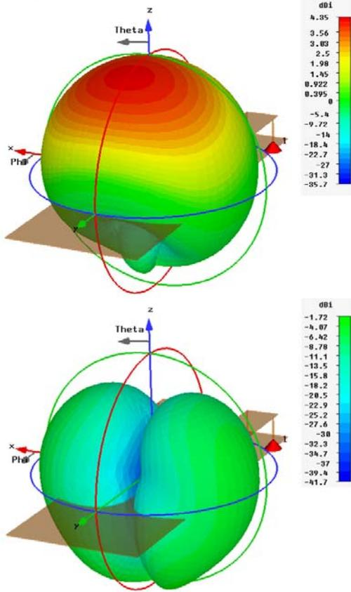
Fig. 7. Vertical (top) and horizontal (bottom) far field components at 2 GHz for in-phase excitation
